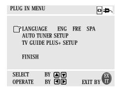
The "Plug In Menu" only appears the first time the TV is plugged in, or after a power interruption of more than 90 seconds.
